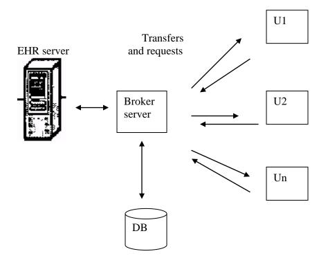
Figure 3. Broker server operation
